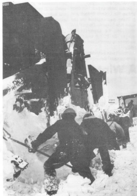
HIGH snowdrifts flanked these engines on a track in Indiana as they were stranded because of a freeze-up (above). Conrail employees (below right) struggle to free a Jordan spreader on an Indiana track after it had derailed while in service pushing snow. The spreader is normally used to grade cuts and fills. Crossbucks (below left) barely stand above dump of snow after plowing.
